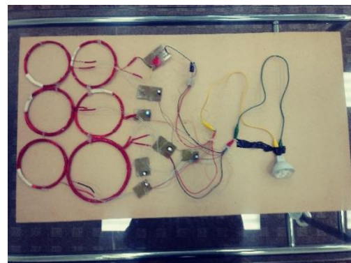
Fig. 15. Photograph of the receiver harvester circuit
